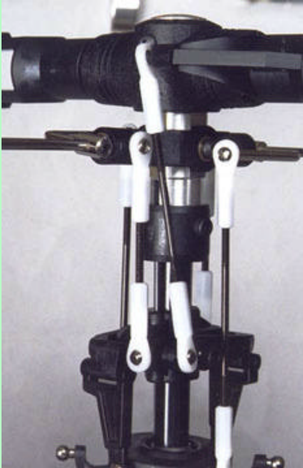
Nice looking head, but watch out for the linkage clash shown at left. If you are using the outer ball position on the seesaw this may not happen
