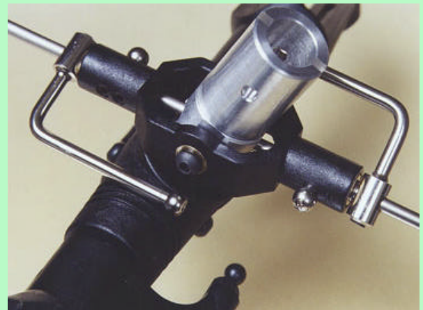
Seesaw arm is plain bushed but shows commendably low slop. The balls on the seesaw have three alternative positions for different response. by way of two holes on one side and one on the other. The seesaw has to be removed and turned over to use the other holes
