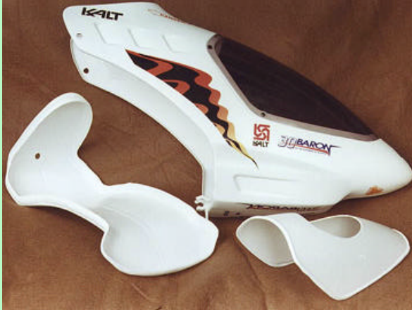
Large lumps have to be cut from the original moulding, but it's pretty easy to do
