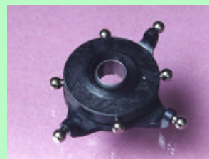
Conventional swashplate has very little slop and is firmly located in the final installation
