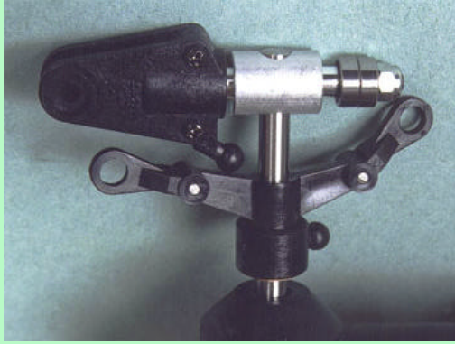
The hub is locked to the shaft with M3 grub screws, which also serve to retain the bearings
