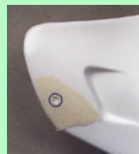
Cutting the grommet holes in the canopy
