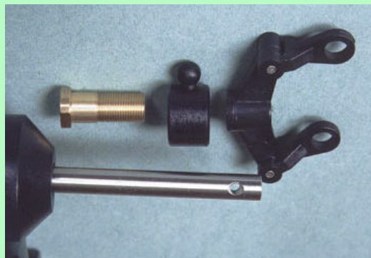
Brass bushed tail slider, with pivoting links, dual ballraces too and below, the very substantial tail drive coupling
