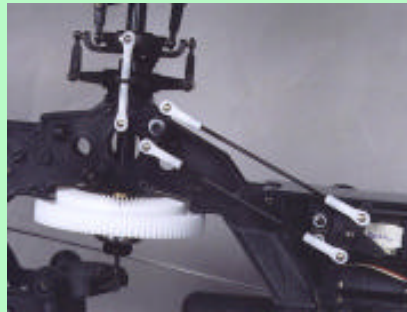
Up to the swashplate; on the left the roll linkage and below, the right hand side of the 30 Baron showing the fully closed loop elevator linkage
