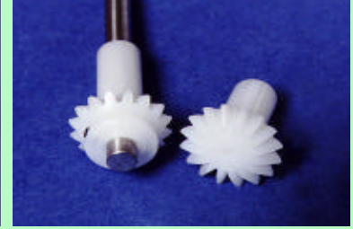
On the left, the brass tube used to push the tail guides in square and right, the tail rotor gears.
