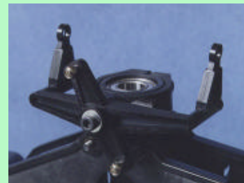
Fore/aft cyclic control lever, it mounts to the ring shaped 'lever bracket'
