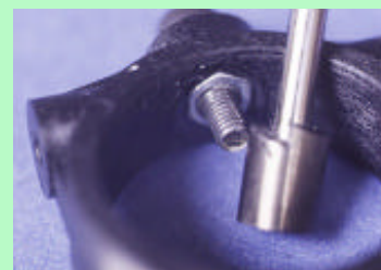
... which doesn't have much thickness for the screw to go into. A counterbore and steel nut is rather more secure
