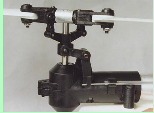
The hub is locked to the shaft with M3 grub screws, which also serve to retain the bearings
