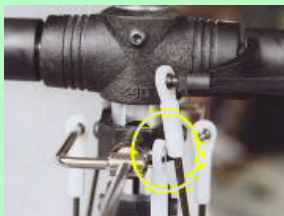
Nice looking head, but watch out for the linkage clash shown at left. If you are using the outer ball position on the seesaw this may not happen
