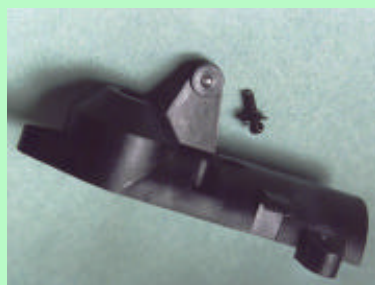
Above, the modified tail rotor servo position and right, the sheared bellcrank screw
