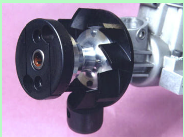
The flywheel won't fit the Irvine 36, but an alternative is available. Lower picture shows the one way start bearing in the clutch
