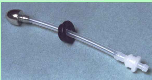
Tank feed is easily accessible, but can cause fuel feed problems. Ingenious grommet for fitting (below) works very well.
