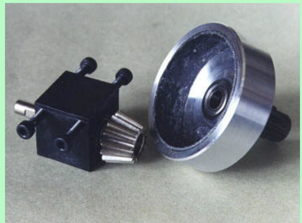
Substantial clutch bell, steel pinion and a very wide main gear
