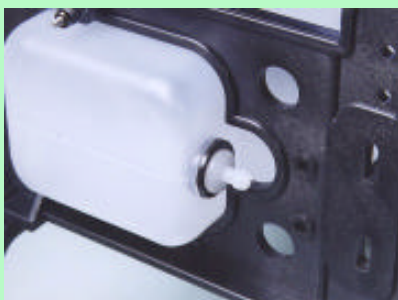
Tank feed is easily accessible, but can cause fuel feed problems. Ingenious grommet for fitting (below) works very well.
