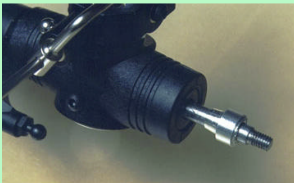
Aluminium damper collars spread the load on the grommet type damper rubbers
