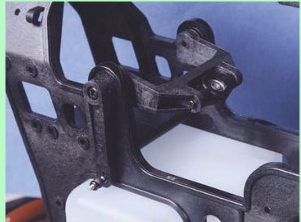
Collective pitch mechanism in place. Note how close the lever is to the chassis
