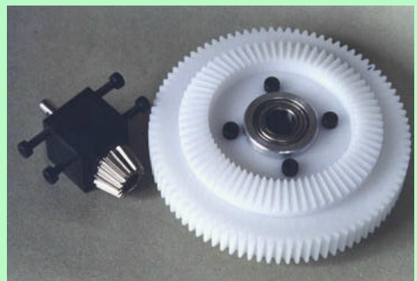
Substantial clutch bell, steel pinion and a very wide main gear
